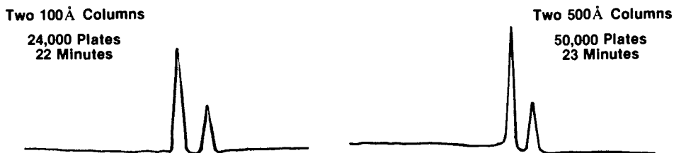
Figure 9. Comparison 100 \text{ \AA} and 500 \text{ \AA} two column sets; plates versus pore amount; Probe Mix 1.
